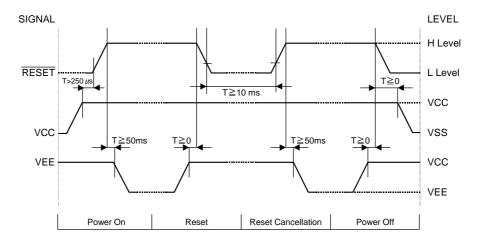
Please maintain the above sequence when turning on and off the power supply of the module. If  $V_{EE}$  is supplied to the module while internal alternate signal for LCD driving (M) is unstable or  $\overline{RESET}$  is active, DC component will be supplied to the LCD panel. This may cause damage to the LCD module.
